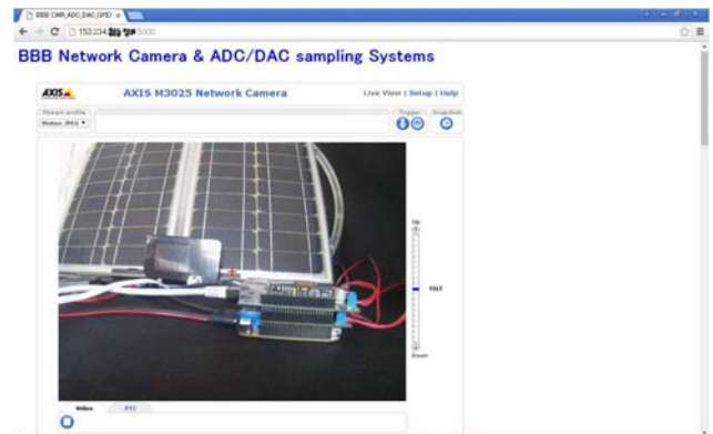
Pic.11 Access screen shot to Network Camera iframe on the BBB Web Server html page through mobile router gateway (port 5000)
