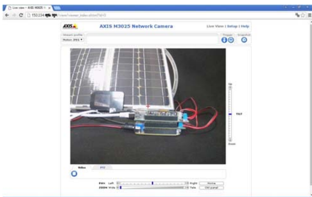
Pic.10 Access screen shot to Network Camera Web Server html page through mobile router gateway (port 80)
